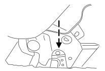
3. Rotate the seat forward until it latches onto the front pin.
